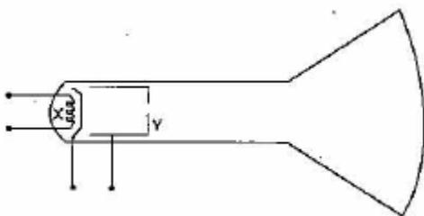
The above diagram shows an electron gun of a hot cathode ray tube,
